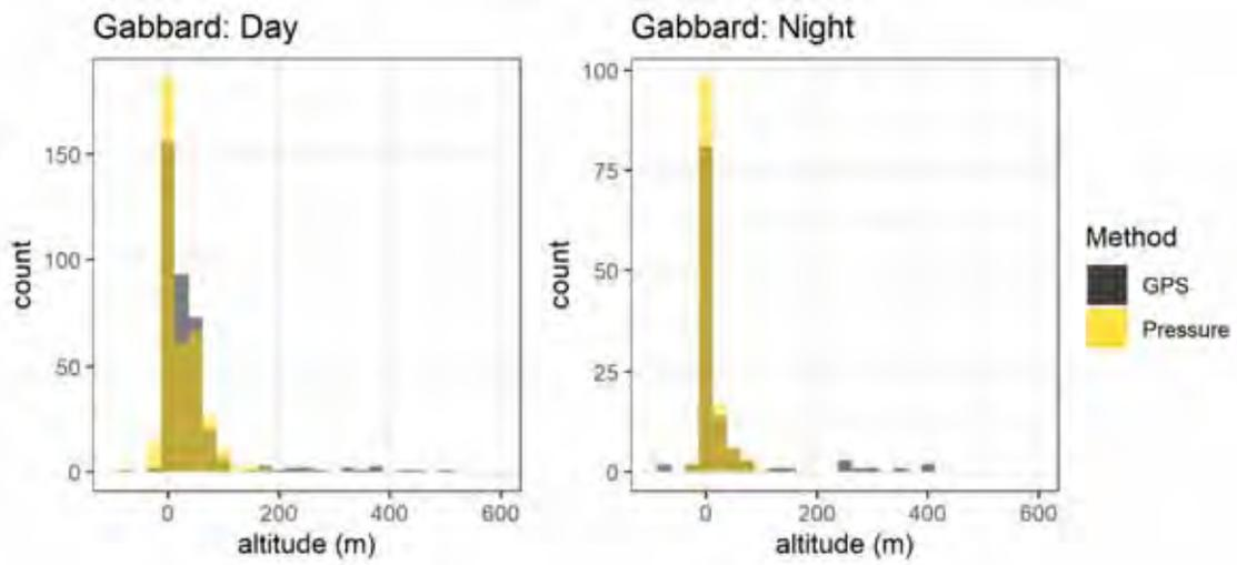
**Figure 4.17** Comparison of GPS (blue bars) and pressure sensor (red bars) derived altitudes within the Greater Gabbard OWF attributed to all fixes at a fix rate of five minutes, split by day and night.
