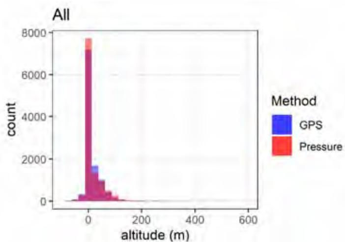
**Figure 4.14** Comparison of GPS (blue bars) and pressure sensor (red bars) derived altitudes attributed to all fixes at a fix rate of five minutes.
