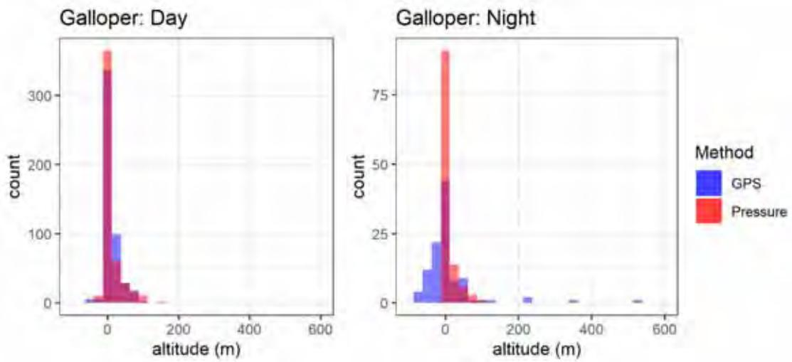
**Figure 4.16** Comparison of GPS (blue bars) and pressure sensor (red bars) derived altitudes within the GWF attributed to all fixes at a fix rate of five minutes, split by day and night.
