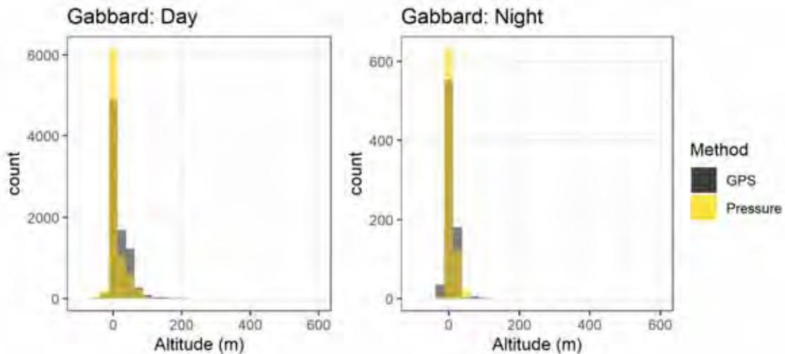
**Figure 4.21** Comparison of GPS (black bars) and pressure sensor (yellow bars) derived altitudes within the Greater Gabbard Wind Farm attributed to all fixes at a fix rate of 5-10 seconds, split by day and night.
