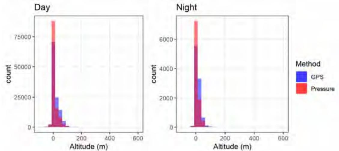
**Figure 4.19** Comparison of GPS (blue bars) and pressure sensor (red bars) derived altitudes attributed to all fixes at a fix rate of 5-10 seconds, split by day and night.
