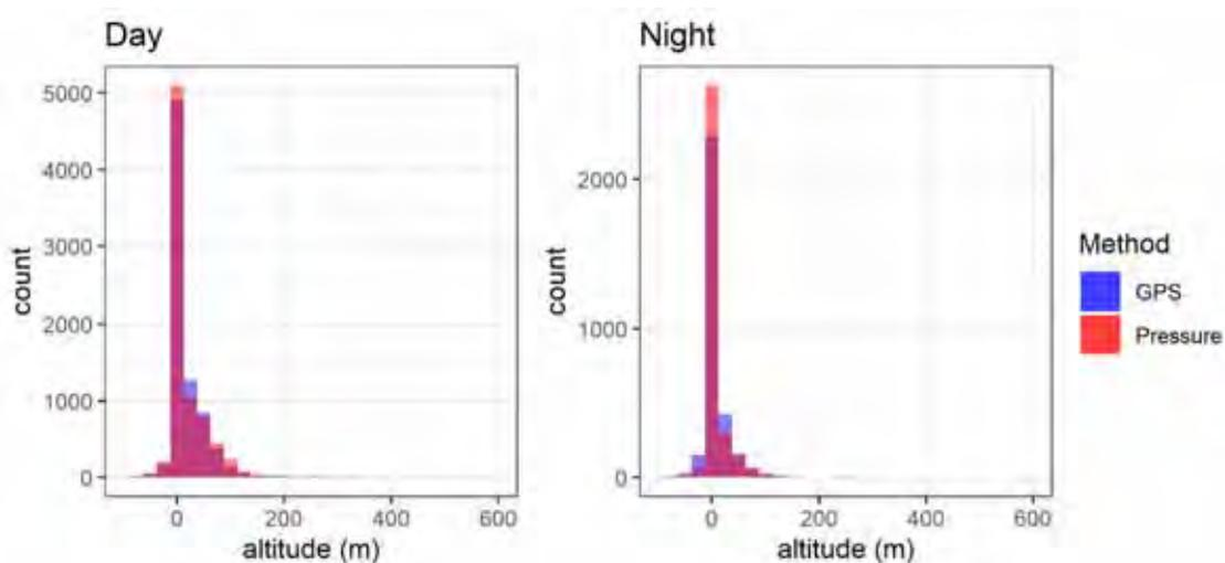
**Figure 4.15** Comparison of GPS (blue bars) and pressure sensor (red bars) derived altitudes attributed to all fixes at a fix rate of five minutes, split by day and night.
