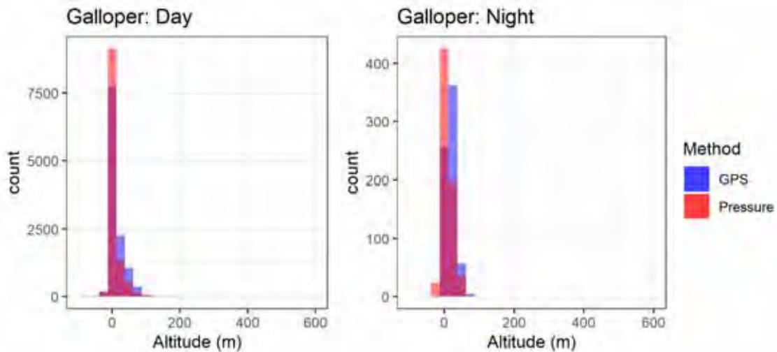
**Figure 4.20** Comparison of GPS (blue bars) and pressure sensor (red bars) derived altitudes within the GWF attributed to all fixes at a fix rate of 5-10 seconds, split by day and night.
