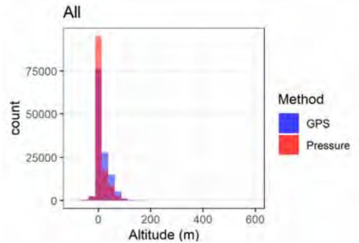
**Figure 4.18** Comparison of GPS (blue bars) and pressure sensor (red bars) derived altitudes attributed to all fixes at a fix rate of 5-10 seconds.
