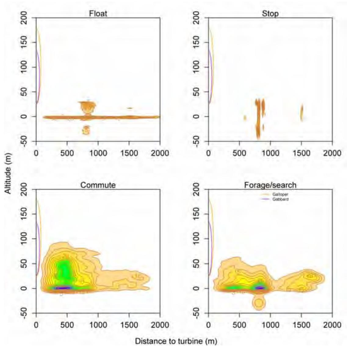
**Figure 4.33** Distribution of Lesser Black-backed Gulls within the Galloper and Greater Gabbard Wind Farms in relation to distance from nearest turbine and altitude, based on data collected at a 5-10 second rate, split by EMbC behavioural state, and as assessed through a kernel density estimation. The three-dimensional rotor swept volume is indicated for the Galloper and Greater Gabbard Wind Farms, respectively.
