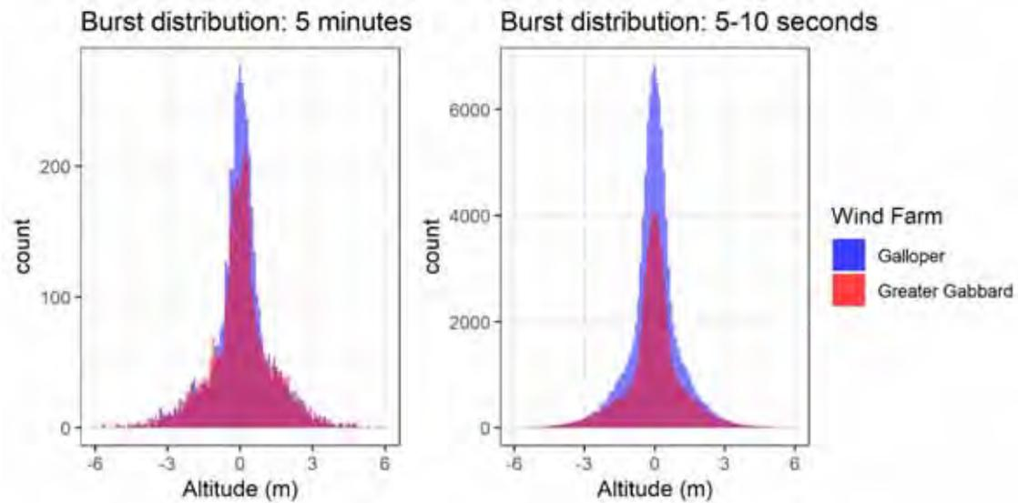
**Figure 4.25** Standard deviations of altitudes produced from pressure burst values (10 per fix) in relation to fix rate, for the GWF (blue) and Greater Gabbard Wind Farm (red).
